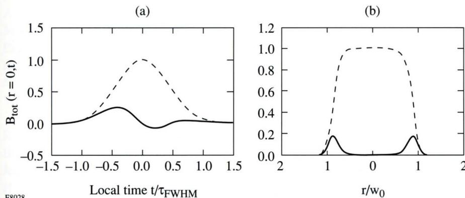
Figure 67.33 Theoretically estimated residual phase after the propagation of a 1-ns pulse with an incident peak  $B$ -integral of unity before (dashed line) and after (solid line) GaAs plate with  $\alpha = 1 \text{ cm}^{-1}$ ,  $L = 2 \text{ mm}$ ,  $I_{\text{inc},0} = 90 \text{ MW/cm}^2$ ,  $\tau_{\text{rel}} = \tau_{\text{FWHM}}/10$ : (a) radial profile at the temporal peak of the pulse; (b) temporal profile through the axis of the beam.
